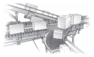
Automated Material Handling Systems ERS Brakes hold rollers and lift mechanisms in place, and lock drive wheels in place.
