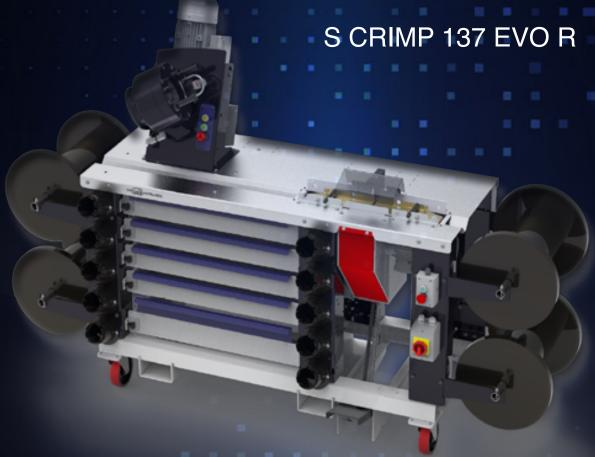
Designed for hoses up to 1.1/4", this version of the "Hose Room on Wheels" combines the precision and efficiency of the S CUT 30 L cutting machine with the convenience and ergonomic design of the S CRIMP 137 EVO R crimping machine, for a versatile and reliable mobile assembly solution.
