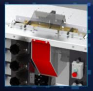
Both models of the "Hose Room on Wheels" come fitted with an integrated version of the S CUT 30 L cutting machine. Fitted with a scalloped blade for efficient, precise cutting with minimal smoke production, the S CUT 30 L also has a built-in dust collector and foot-pedal.
