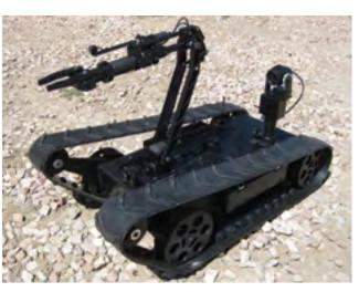
Military and Law **Enforcement Robots (left)** An industry leader in defense robotics utilized two Polyclutch slip clutches in each robot arm for overload protection.
