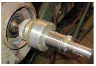
**Mechanical Safety** - The V-Series Slipper provides overload protection and increases operator safety to this manual cutting tool. This mechanical slip clutch limits the amount of torque that is transferred to the cutting tool, making this a safer operation for the user.
