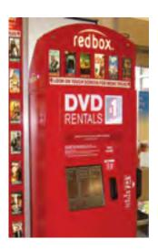
**Retail Vending Kiosks (right)** A Polyclutch protects this machine against any type of overload or jamming during the process of dispensing a DVD
