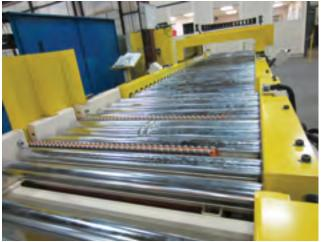
Conveyors (left) Polyclutch® slip clutches offer an added level of safety and protection to both the machine and its operators.
