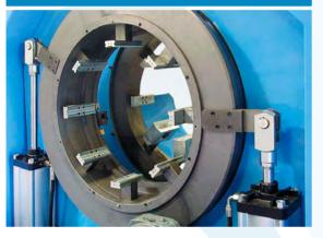
The automatic pneumatic clamping systems are fixing the pipe concentric. The machining is performed between the both clamping systems.
