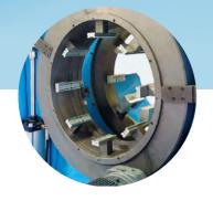
The machine is designed with a double external clamping of the tubes upstream and downstream of the internal part of the machine.
