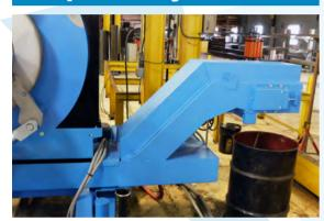
The option chips conveyor can be used on all versions of the CTA. This option enables to increase the productivity rate as all the chips pro-duced during a machining cycle are re-moved automatically.
