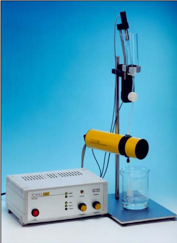
Particle Analysis System for Fluids FAS 362
