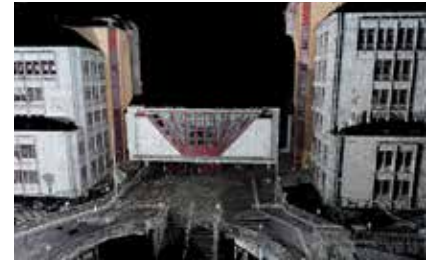
automatically cleaned-up point cloud
