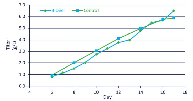
The BIONe single-use bioreactor system effectively eliminates the time, risk, and costs associated with cleaning, assembling, and autoclaving non-disposable bioreactors. The BIONe achieved comparable growth profiles and recombinant protein production relative to a glass vessel bioreactor. Similar performance attributes in these key areas demonstrate the BIONe's utility as a robust model for bioprocess development.
