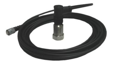
It is very easy to mount, both for short duration measurements, (it has several accessories available for magnetic or contact fixing) and in permanent installations (removable mounting stud). The AC001 is supplied with a BNC connector ended cable to connect it to instruments with ICP<sup>©</sup> devices input.
