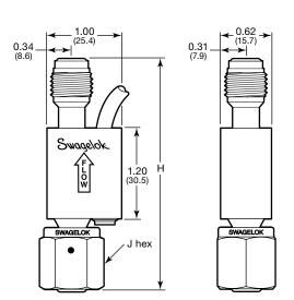
Dimensions shown with Swagelok tube fitting nuts finger-tight.
