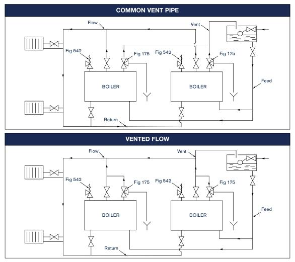
In both types of installation, there must be no isolating valve fitted between the Fig 175 and the boiler, vent pipe or drain.
